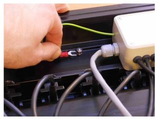
3. Connect the wire to the grounding pin.
