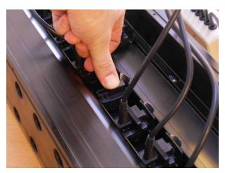
3. Then push down the sensor, so the sealing rings are sealed tight.
