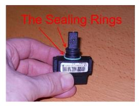
7. Check that the sealing ring is not left in the sensor hole on the manifold.
