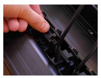
4. Place the clips over the sensor, so that the socket is accessible.
