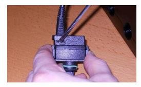
5.Gently unsnap the wireplug with a small straight notch screwdriver in each side.
