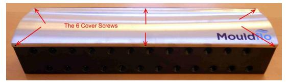
1. Remove the 6 cover screws. (M4x6) then lift off the cover.
