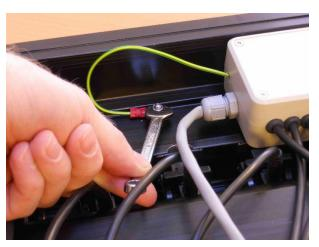
4.Refit the M4 nut, so the wire does not come off.
