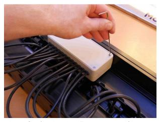
2. Refit the 2 M3x45 countersunk mounting screws.
