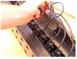
2.Release the clips manually or with a small plier.
