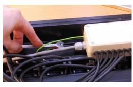
2. Remove the nut, holding the ground wire (M4).
