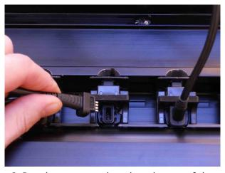
6.Gently connect the plug, be careful not to bend any of the sensor pins in the socket.
