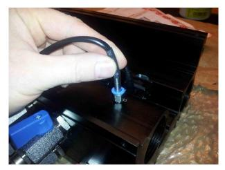
5. Push the temperature sensor into the blue fitting, an try to pull it to
