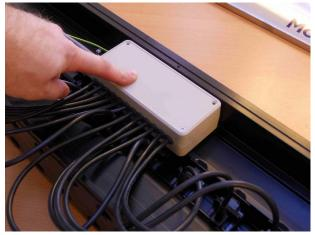
1. Place the sensor box over the mounting holes.
