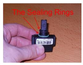
7. Make sure the sealing rings are not left in the sensor
