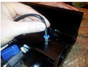
5. Push the temperature sensor into the blue fitting,
