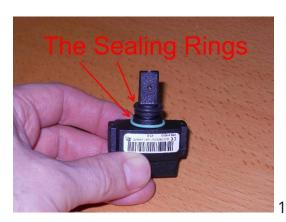
1. Make sure that both sealing rings are on the new
