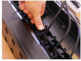
3. Then push down the sensor, so the sealing rings are
