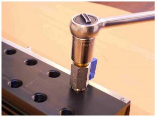
2. Tighten the valve so the valve handle is not in the way of the other valves.
