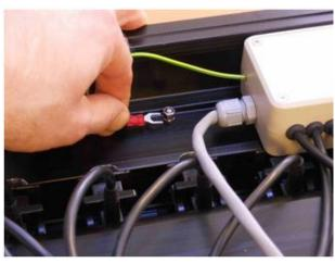
3. Connect the wire to the grounding pin.
